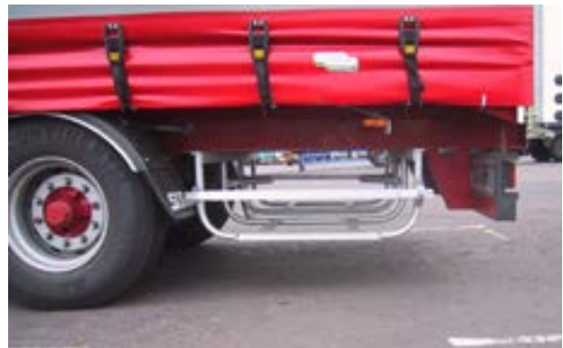
Fig no. 2 Spare wheel carrier lower than tail bar
