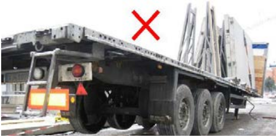
Incorrect weight balance, fig no. 36
