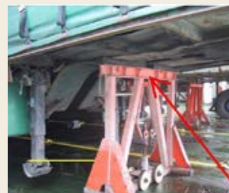
Fig no. 10 An example of a trestle in place correctly supporting a semi-trailer
