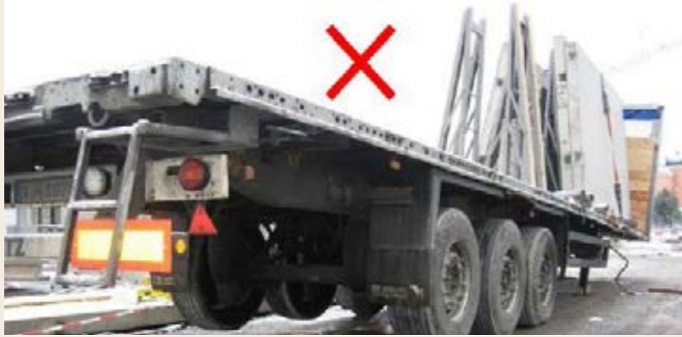
Incorrect weight balance, fig no. 36
