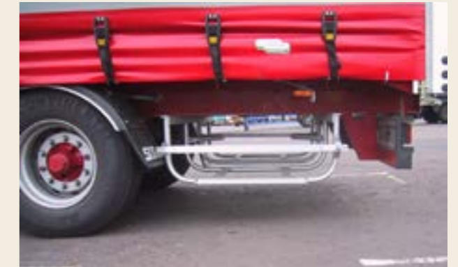
Fig no. 2 Spare wheel carrier lower than tail bar
